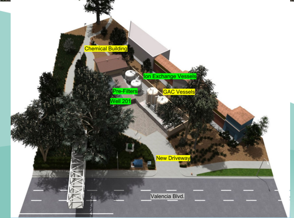
Well 201 Groundwater Treatment
