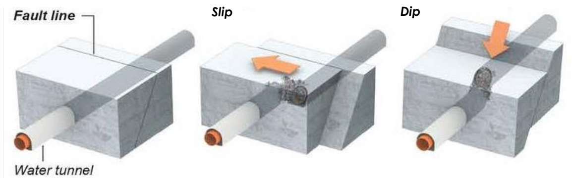
FIGURE 8. How Ground Displacement Can Sever Pipes
