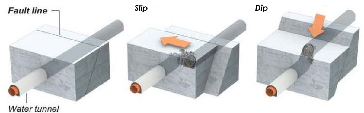
FIGURE 8. How Ground Displacement Can Sever Pipes
